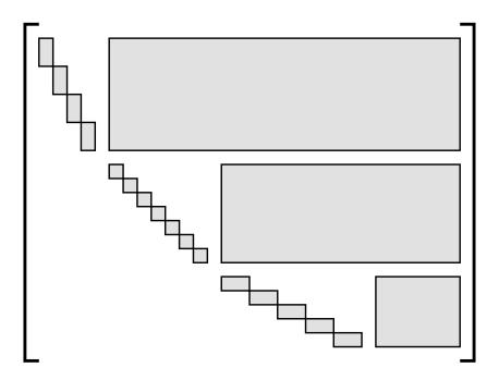
*Strongly filtered matrix*: block triangular where the diagonal blocks are themselves block decomposed.
